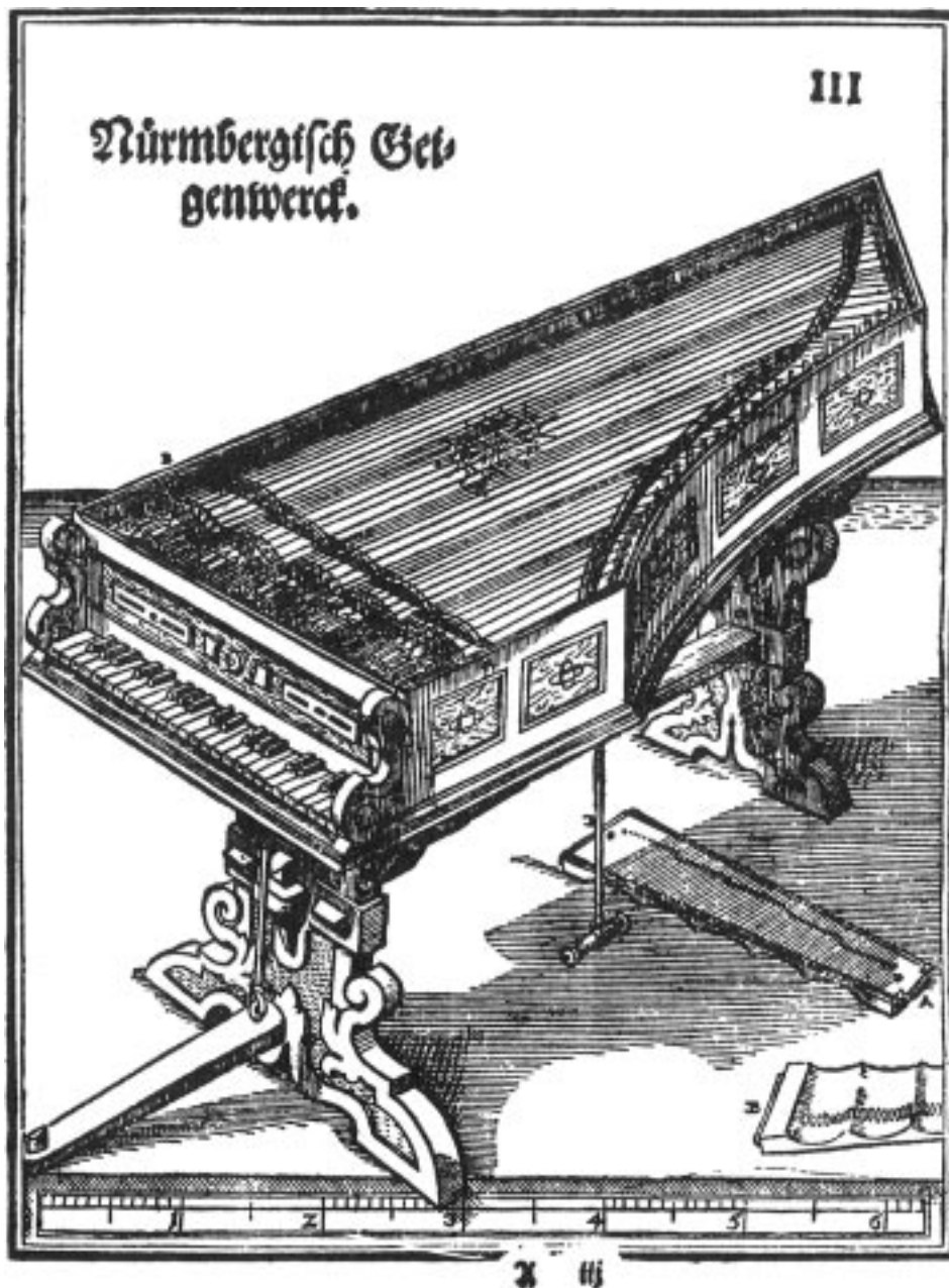
Figure 1 — Woodcut of Haiden's Geigenwerk from Praetorius, Theatrum instrumentorum , 1620. The pinblock is in five rounded sections, corresponding to the five rosined wheels, which revolve by use of the treadle mounted on the front leg. The instrument's name comes from the fact that the wheels, like violin bows, make the strings vibrate by friction, and Geige is the German word for violin.
